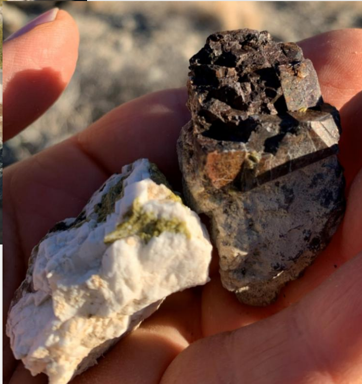
Distal epidote (green mineral) and vesuvianite (reddish-brown crystals) alteration south of Gold Bug.
