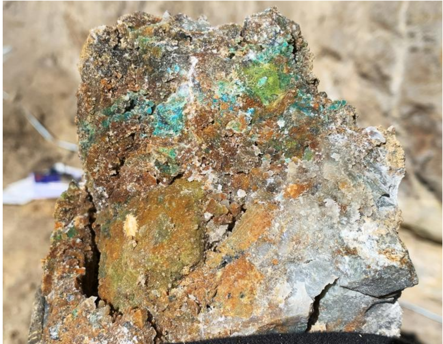
Example of vein material from Golden Bomber shows it is a low sulphidation (LS) epithermal vein based on the chalcedonic form of quartz.
